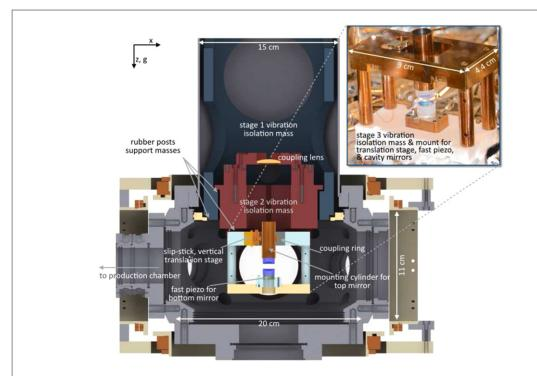
**Figure 3.** Computer rendering of a section-view of the science chamber showing the cavity mount, vibration isolation stages, and invacuum coupling lens. Note, colors do not reflect actual material color. Inset: photograph of cavity holder outside of vacuum, including single-crystal PZT, mirrors, and slip-stick translation stage.
