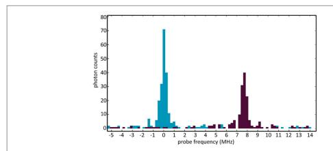
**Figure 7.** Single-shot data of bare cavity resonance (left, blue) and dispersively coupled cavity resonance (right, purple) versus frequency for a single-mode configuration with L>R, as shown in figure 4(e). The coupled resonance is shifted by  $\delta\omega_c^{\rm SM}=7.66(2)$  MHz. Data taken for  $N=2.0(2)\times 10^5$  atoms and  $\Delta_A=\omega_l-\omega_h=8.7(1)$  GHz. The sweep rate is 20 MHz/40 ms.
